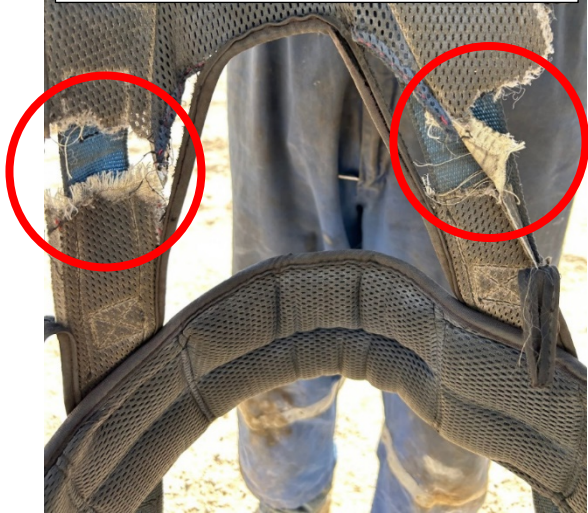
Tension forces applied to the safety harness deployed the impact indicators as designed (like impact loading in the event of a fall).
